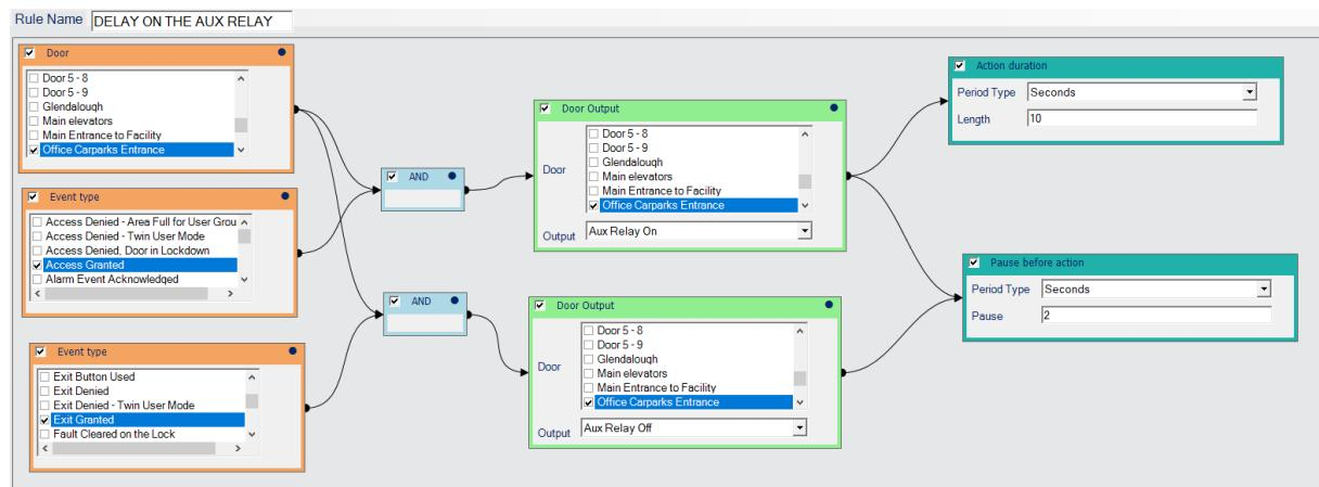
In the above example, if an access/exit granted occurs on door “Office Carparks Entrance” the aux relay fires 2 seconds after the main relay using the “Pause Before Action” function. Using the “Action duration” function the installer can define how long the activation lasts.
