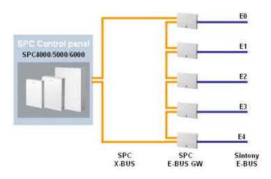
"This is achieved by installing an SPC E-Bus Gateway which allows newly installed SPC system panels communicate with the Sintony E-Bus network and its E-Bus devices."
