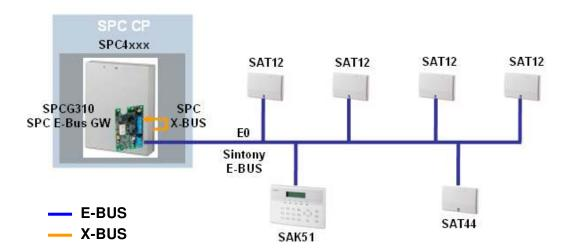
In the above diagram the SPC E-Bus GW (SPCG310) is shown mounted in the SPC control panel housing. It can also be mounted in Sintony SAH14 housing or in external power supply housing.
