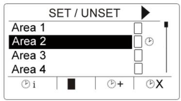
When the timer displays next to an area, 3 timer symbols display above the soft keys:
