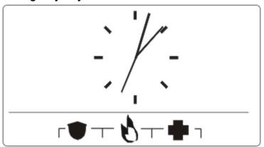
Depending on configuration, emergency keys are displayed. A simultaneous pressing of the keys activates an emergency call.
